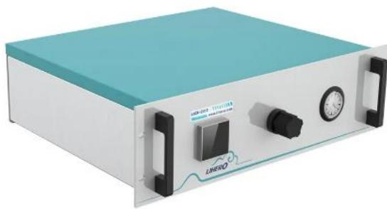
The air compressor of this product compresses the external air, and after the dew point is reduced to -20°C through the polymer dehumidification tube, the high-temperature catalytic furnace performs high-temperature oxidation and decomposition of CO, hydrocarbons, and ozone, and then adsorbs SO<sub>2</sub>, nitrogen oxides, etc. through the filter material, and finally outputs zero-level air with stable pressure through the pressure regulating valve.
