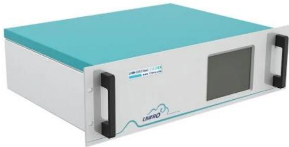
This product uses a flow controller based on the laminar differential pressure measurement principle to control the raw gas and dilution gas. Since the controller has its own temperature and pressure compensation, it does not need to control the external environment temperature and gas pressure to achieve high-precision control of the single-channel gas flow.
